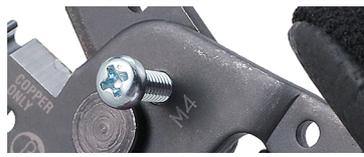
Can cut the screw thread to make the length shorter. Good for circuit board fixing during electronic component assembly.
