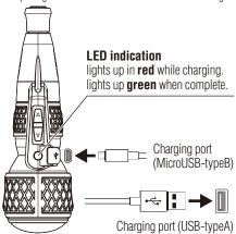
2) Insert the other end of the USB charging cable to a USB port designated in the specifications (commercially available AC adapters, PCs. mobile batteries. etc.). The charging lamp lights up and the charging starts. While charging the battery, the charging lamp lights red. When charging is complete, the charging lamp lights green.
