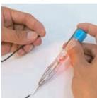
Continuity check of a wiring circuit Make sure that no power is applied to the circuit before checking continuity.
